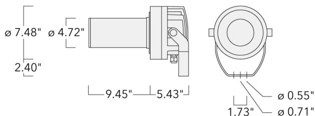
IP66. Class I. IK07. Marine-grade, die-cast aluminum alloy. 5CE superior corrosion protection including PCS hardware. Silicone CCG® Controlled Compression Gasket. Safety glass lens. One cable gland, second gland for through wiring on request. PMMA LED lens array. Integral driver, thermally separated. Factory-installed LED circuit board. Tunable White technology. LED board can be removed for upgrading. DMX Interface.
