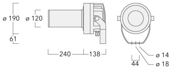
IP66, Class I. IK07. Marine-grade, die-cast aluminium alloy. 5CE superior corrosion protection + primer including PCS hardware. Silicone CCG® Controlled Compression Gasket. Safety glass lens. One cable gland. Second gland for through wiring on request. PMMA LED lens array. Factory installed LED circuit board. LED board can be removed for upgrading. Integral EC electronic converter, thermally separated. DALI interface.
