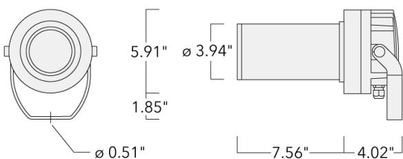
IP66, Class III. IK05. Marine-grade, die-cast aluminum alloy. 5CE superior corrosion protection including PCS hardware. Silicone CCG® Controlled Compression Gasket. Safety glass lens. One cable gland. Second gland for through wiring on request. Integral driver in separate driver box (medium), prewired. OLC® One LED Concept. Factory installed LED circuit board. Color Changer technology. DMX interface.
