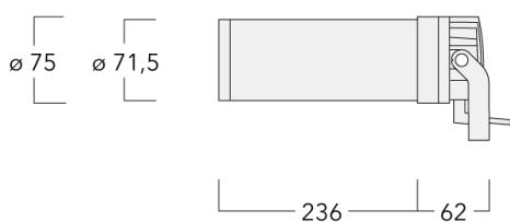
IP66, Class III. IK07. Marine-grade, die-cast aluminium alloy. 5CE superior corrosion protection including PCS hardware. Silicone CCG® Controlled Compression Gasket. Safety glass lens. Electronic control gear in separate gear box (constant current), prewired. Gearbox to be ordered separately. One factory installed flange plug M8 x 1.5. Cable length 10 ft. CAD-optimised optics for superior illumination and glare control. Factory-installed LED circuit board.
