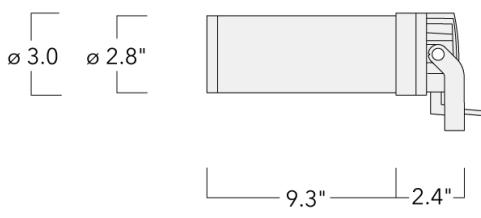
IP66, Class III. IK07. Marine-grade, die-cast aluminium alloy. 5CE superior corrosion protection including PCS hardware. Silicone CCG® Controlled Compression Gasket. Safety glass lens. Electronic control gear in separate gear box (constant current), prewired. Gearbox to be ordered separately. One factory installed flange plug M8 x 1.5. Cable length 10 ft. CAD-optimised optics for superior illumination and glare control. Factory-installed LED circuit board.
