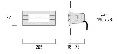
A pre-installation blockout is available and recommended for mounting in concrete walls. To be ordered separately.
