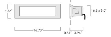
IP66. Class I. IK10. Marine-grade, die-cast aluminum alloy housing, with polished stainless-steel frame. 5CE superior corrosion protection including PCS hardware. Silicone CCG® Controlled Compression Gasket. Opal polycarbonate main lens. Two cable entries. Integral driver. Factory-installed LED circuit board. 0-10V Dimming standard.
