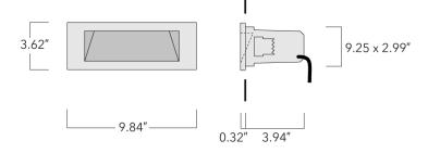
IP66. Class I. IK10. Marine-grade, die-cast aluminum alloy. 5CE superior corrosion protection including PCS hardware. Silicone CCG® Controlled Compression Gasket. Safety glass lens. Two cable entries. Integral driver. Factory-installed LED circuit board. 0-10V Dimming standard. ETL, UL-1598, CSA-C22.2#250.0. Suitable for Wet Locations.
