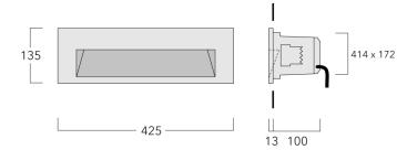
A pre-installation blockout is available and recommended for mounting in concrete walls. To be ordered separately.
