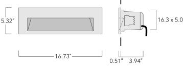
IP66. Class I. IK10. Marine-grade, die-cast aluminum alloy. 5CE superior corrosion protection including PCS hardware. Silicone CCG® Controlled Compression Gasket. Safety glass lens. Two cable entries. Integral driver. Factoryinstalled LED circuit board. 0-10V Dimming standard.
