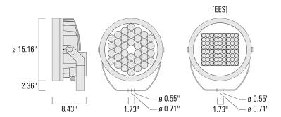
IP66. Class I. IK07. Marine-grade, die-cast aluminum alloy. 5CE superior corrosion protection including PCS hardware. Silicone CCG® Controlled Compression Gasket. Safety glass lens. One cable gland, second gland for through wiring on request. CAD-optimized optics for superior illumination and glare control. Integral driver, thermally separated. OLC® One LED Concept. Factory-installed LED circuit board. DMX interface.
