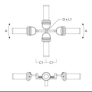
TA4 Mounting bracket, quad (Ø 108 x 147-0100  $\pm 90^{\circ}$  650 108 x 200 24.20 108 x 200 200)
