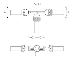
TA3 Mounting bracket, triple (Ø 108 x 147-0098  $\pm 90^{\circ}$  650 108 x 200 24.20 108 x 200 200)
