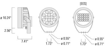
IP66. Class I. Marine-grade, die-cast aluminum alloy. 5CE superior corrosion protection including PCS hardware. Silicone CCG® Controlled Compression Gasket. Safety glass lens. Two cable glands; one for power, one for DMX. CAD-optimized optics for superior illumination and glare control. Integral driver, thermally separated. OLC® One LED Concept. Factory-installed LED circuit board. DMX interface.
