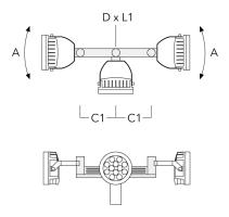
TA3 Mounting bracket, triple (Ø 4.25
