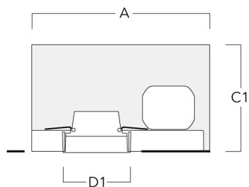
**Ceiling Luminaires****Installation blockout, flush with shadow line**
