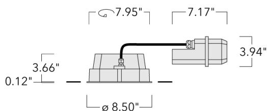
IP66, Class I. IK07. Marine-grade, die-cast aluminum alloy. 5CE superior corrosion protection including PCS hardware. Silicone CCG® Controlled Compression Gasket. Safety glass lens. Separate IP66 driver housing. CAD-optimized optics for superior illumination and glare control. OLC® One LED Concept. Factory installed LED circuit board. 0-10V Dimming comes standard with luminaire.
