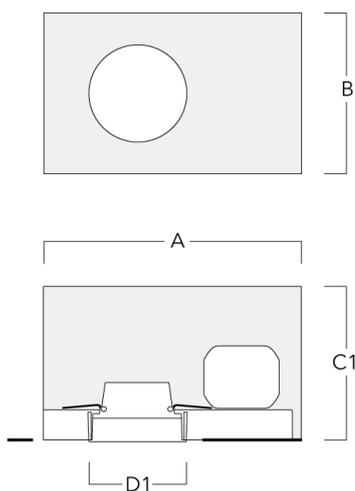
**Installation blackout, flush with shadow line**
