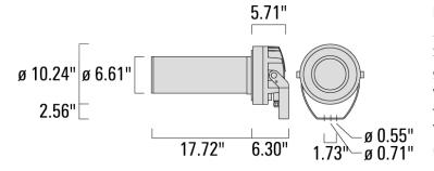
IP66. Class I. IK07. Marine-grade, die-cast aluminum alloy. 5CE superior corrosion protection including PCS hardware. Silicone CCG® Controlled Compression Gasket. Safety glass lens. One cable gland, second gland for through wiring on request. PMMA LED lens array. Integral driver, thermally separated. Factory-installed LED circuit board. Tunable White technology. LED board can be removed for upgrading. DMX interface.
