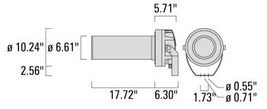
IP66. Class I. IK07. Marine-grade, die-cast aluminum alloy. 5CE superior corrosion protection including PCS hardware. Silicone CCG® Controlled Compression Gasket. Safety glass lens. One cable gland, second gland for through wiring on request. PMMA LED lens array. Integral driver, thermally separated. Factory-installed LED circuit board. Tunable White technology. LED board can be removed for upgrading. DMX interface.
