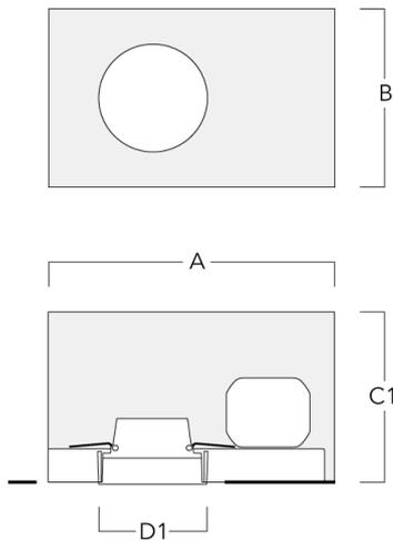
**Installation blackout, flush with shadow line**
