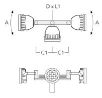
TA3 Mounting bracket, triple (Ø 4.25 147-0098  $\pm 90^{\circ}$  25.59" 4.25 x 8 53.35 lbs 108 x 200 x 8)
