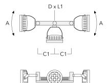
TA3 Mounting bracket, triple (Ø 4.25 147-0098  $\pm 90^{\circ}$  25.59" 4.25 x 8 53.35 lbs 108 x 200 x 8)
