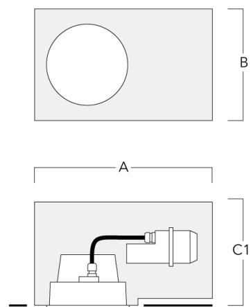
**Installation knockout, flush with shadow line - reduced depth**
