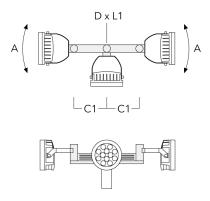
TA3 Mounting bracket, triple (Ø 4.25
