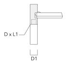
Pole bracket RM2-76, double for 105-9850 114 76 x 80 1.30 mounting on AMF-C poles
