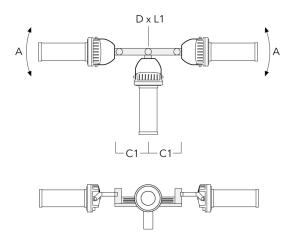
TA3 Mounting bracket, triple (Ø 4.25 147-0098  $\pm 90^{\circ}$  25.59" 4.25 x 8 53.35 lbs 108 x 200 x 8)
