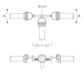
TA3 Mounting bracket, triple (Ø 4.25
