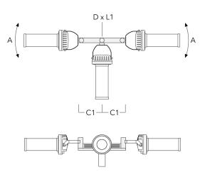
TA3 Mounting bracket, triple (Ø 4.25 147-0098 ±90° 25.59" 4.25 x 8 53.35 lbs 108 x 200 x 8)
