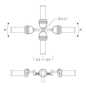
TA4 Mounting bracket, quad (Ø 4.25 147-0100  $\pm 90^{\circ}$  650 4.25 x 8 53.00 108 x 200 x 8)
