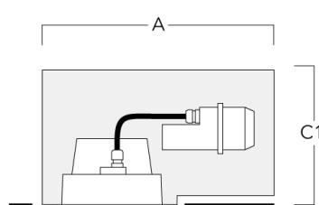
**Installation blockout, flush with shadow line - reduced depth**
