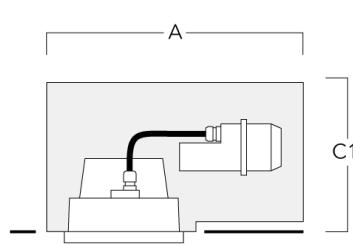
**Installation blockout, flush with shadow line - reduced depth**
