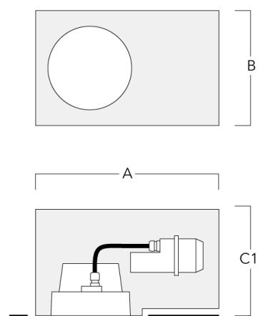
**Installation breakout, flush with shadow line - reduced depth**
