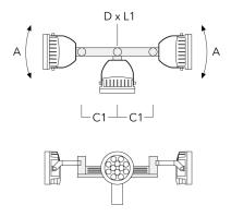
TA3 Mounting bracket, triple (Ø 4.25
