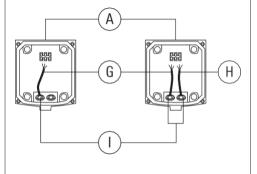
6) Luminaire is also supplied with accessories to suit a variety of cable types. Unscrew membrane sprout(s) I and place packing ring L (for cable diameters 7-9.5mm) or packing ring M (for TPS cable), depending on cable type. Thread cable G through, and screw down pressure screw N.
