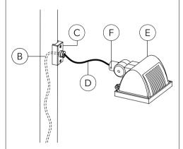
Turn luminaire E towards object to be illuminated. Ensure slipfitter is properly seated on pivot, then tighten screws F.
