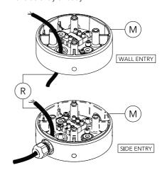
For side entry installations, replace the pre-installed plugs with provided cable glands as required.
