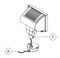
Turn luminaire towards object to be illuminated. Ensure slipfitter is properly seated on pivot, then tighten screws F.
