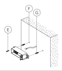
To fix wall flange A, insert and tighten screws E. The orientation of wall flange A detemines orientation of luminaire (up or down)
