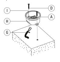
Ensure that all surfaces are clean and dry. Attach terminal connector C and position luminaire over mounting flange A. Turn luminaire towards object to be illuminated. Tighten screw B.
