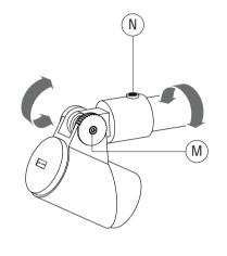
10) For accessory Linear Spread Lens IO-180 or glare shield ES-FLC301: Turn frame **0** to set desired orientation of light or shielding.
