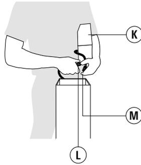
11) Hold luminaire head **K** under arm, reconnect plug **L/M** and place luminaire head **K** on profile **A** and check for alignment.
