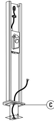
7) Pull cable through centre-hole and screw flange plate **C** with M12 bolts to the planted root (optional).
