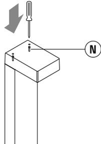
12) Tighten recessed screws **N** gradually in alternating sequence (6 Nm) with Torx 30. Return countersunk screws **J** into head and tighten.
