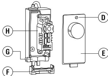
8) Loosen screws **D** from the earth cable connecting box and remove cover **E**.
