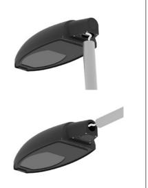
3. Place the luminaire on the pole or outreach. Tighten the M8 grub screws to 5Nm and ensure the luminaire is securely attached to the pole or outreach.
