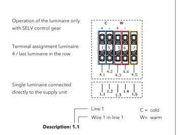
The supply unit 139-6978 is designed for the operation of 1 – 4 luminaires in a row and a distance from the supply unit to the last luminaire of max. 80 ft. FLC210-TW: max. 1300mA ; FLC210-TW PP: max. 500mA
