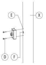
Set and fix column fitter B in position. Insert and tighten screws D.
