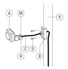
4) Feed cable C from luminaire A through pivot I on column X, while connecting luminaire A with column fitter B by sliding slipfitter H over pivot I. Turn luminaire A towards object to be illuminated. Ensure slipfitter H is properly seated on pivot I, then tighten screw M.
