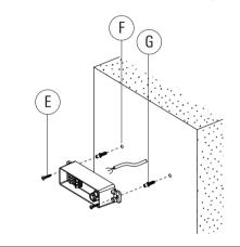
To fix wall flange A, insert and tighten screws
