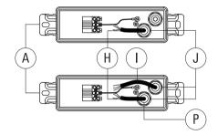
The pre-installed packing ring P is suitable for cable diameters 7 to 9.5 mm and TPS cable to suit 1.5 - 2.5mm.
