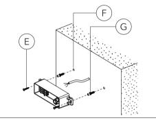
6) To fix wall flange A, insert and tighten screws E. The orientation of wall flange A determines orientation of luminaire (up or down)
