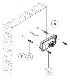
5) Feed mains supply cable G (and second cable H for through wiring, if required) through cable entry J, while setting wall flange A in position. The pre-assembled cable entry  $\bf J$  and packing ring  $\bf I$  are suitable for cable diameters of 0.276 - 0.374 in. For larger cable diameters of 0.354 - 0.472 the enclosed cable entries must be used.
