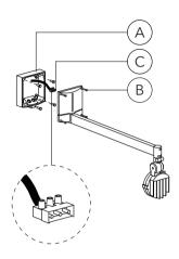
Determine position for fixing screws D. Drill relevant holes E and insert nylon plugs F.
