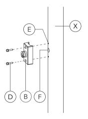
3) Set and fix column fitter **B** in position. Insert and tighten screws **D**.
