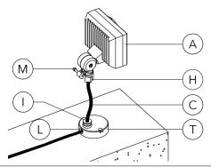
5) Clamp strain relief clip **K** on cable **C** and press into hole **L** of flat surface fitter **T**. Ensure the strain relief clip **K** is properly placed in position to lock the cable.
