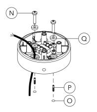
4) Feed cable S from luminaire through pivot of cover L. Connect cable R and S to terminal block T according to wiring shown in separate luminaire installation instruction.
