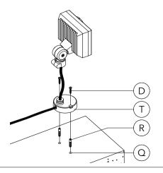
4) Loosen screw M on slipfitter H (do not turn it out) until splipfitter can be opened. Connect luminaire A with flat surface fitter T by sliding slipfitter H over pivot I, while pulling luminaire cable C through hole L and turning luminaire A towards object to be illuminated. Ensure slipfitter H is properly seated on pivot I, then tighten screw M.
