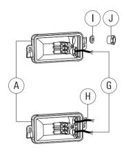
The pre-installed packing ring I is suitable for cable diameters 7 to 9.5 mm.
