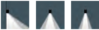
[R45] Rectangular 'side throw' [M] Symmetric, medium beam [N] Symmetric, narrow beam
