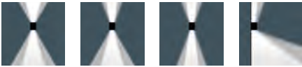
[M/M] Medium beam, up and down [N/M] Narrow beam up, medium beam down [N/N] Narrow beam, up and down [E/A60] Narrow beam up and 'forward throw' down
