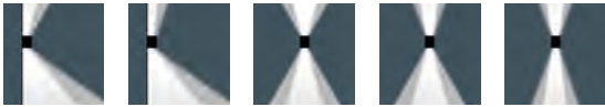
[M/R45] Medium beam up, 'side throw' down [N/R45] Narrow beam up, 'side throw' down [M/M] Medium beam, up and down [N/M] Narrow beam up, medium beam down [N/N] Narrow beam, up and down
