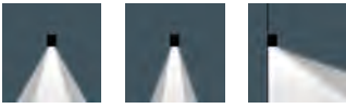
[M] Symmetric, medium beam [N] Symmetric, narrow beam [A60] Asymmetric 'forward throw'
