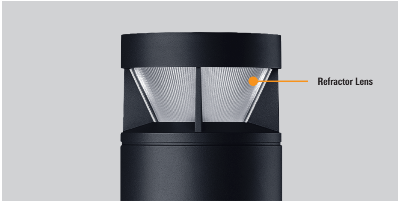
KTX200/KTY200 [C60]. This CAD raytracing simulation demonstrates the controlled downward light distribution. The refractor lens simultaneously reduces surface brightness and provides a limited vertical illuminance component – facilitating facial recognition.
