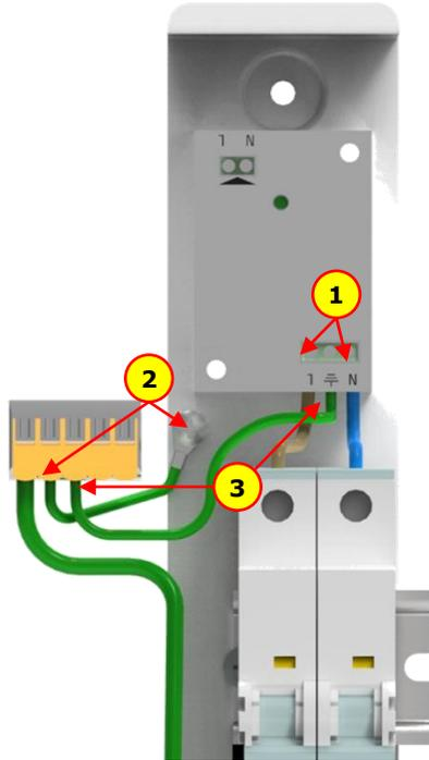
Connect Live and Neutral from MCB to unprotected side of supplied SPD (1), SPD should be earthed to the tray (2,3).
