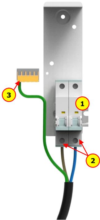
Attach DIN rail and MCB\* (not supplied) to SPD tray (1) and terminate sub circuit leads accordingly(2,3).
