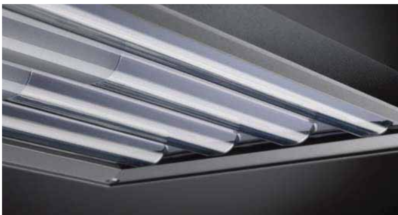
The contour of the main lens follows the shape of the individual LED lens, thereby minimising internal reflections within the luminaire.
